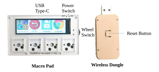
As shown in the diagram above, On top of the device there are (from left to right): a Type-C USB port and the Power switch (slide right to turn on).
